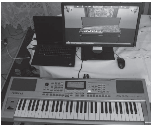
Figure 2: The runtime environment of a virtual model of the clavichord interacting with the MIDI keyboard: MIDI Keyboard Roland EXR-3, a Dell laptop, 23 'Dell multitouch monitor.
